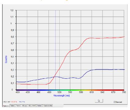
The spectral diagram shows the reflectance data of the standard and the sample in the spectral range from 400 to 700 nm.
