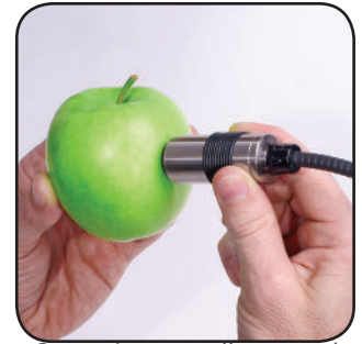
Our unique small external standard 45°/0° probe head
