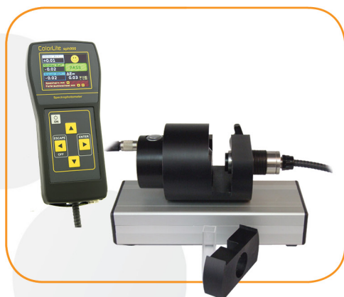
MA35-UK - used for transmission measurements
