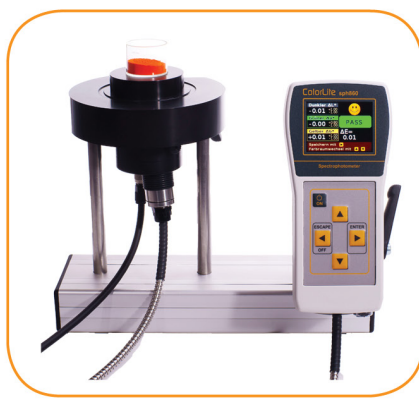
MA35-UK on a Stand for powder measurements
